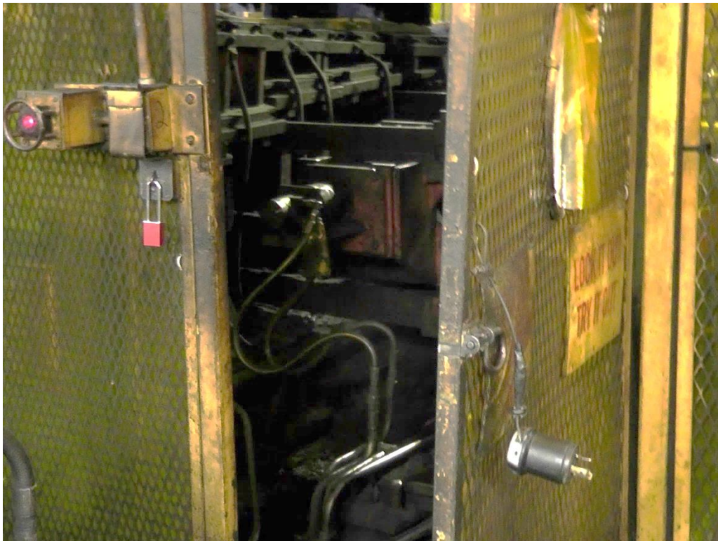
Cord connector used to “interlock” access to machinery.
